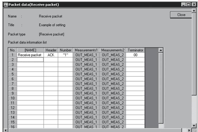
(3) Receive (specified length) packet setting example (Fixed data)
