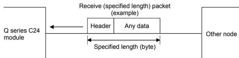
\*1: Any data indicates the data located behind header of the packet sent from other node, or between the header and end judgment data. This data can be omitted. Fixed data and output variables are used as any data when receiving data.
