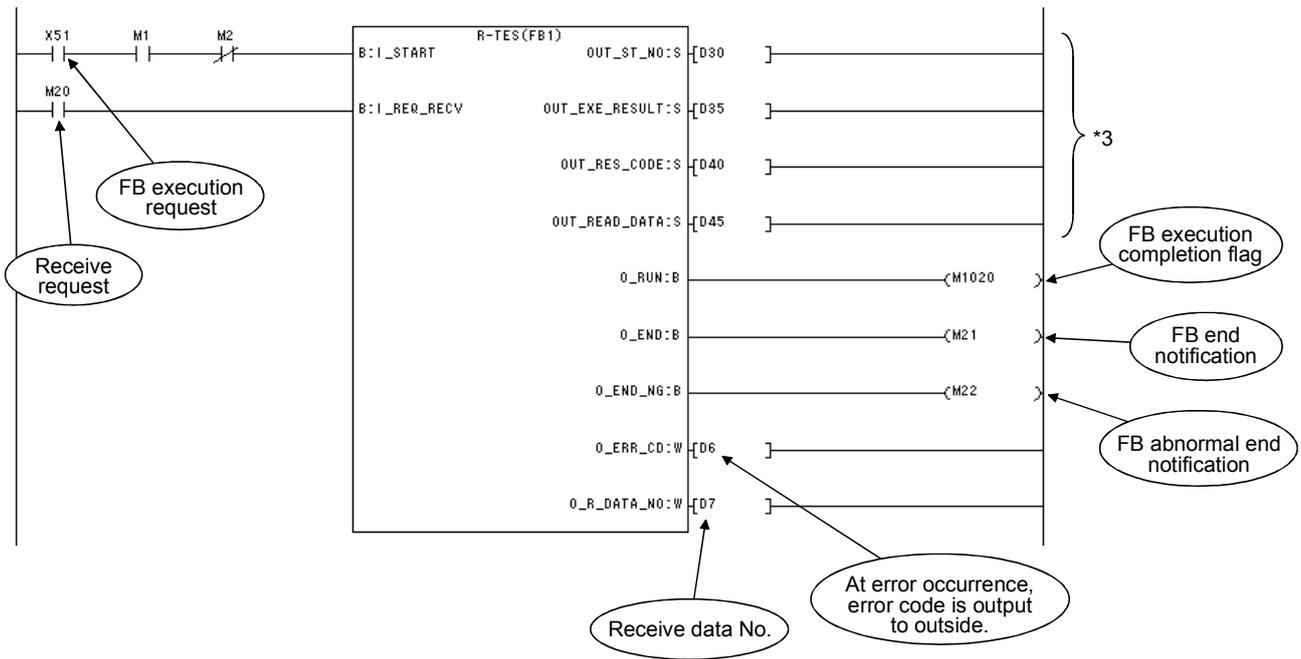
\*3: Variables used when output variables are specified by the user in the packet construction information
