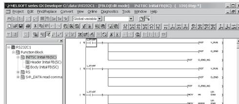
The protocol FB is inserted into the <<FB>> tab.
