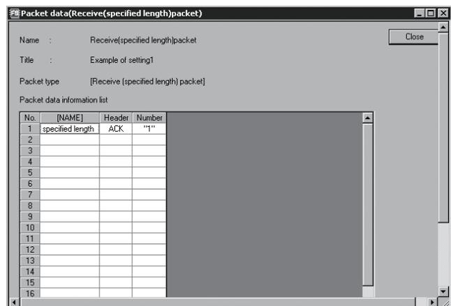
(4) Receive (specified length) packet setting example (Variable data)
