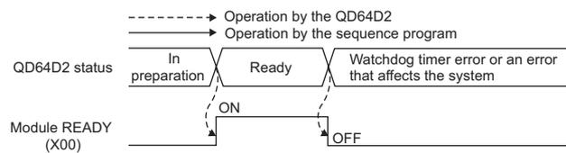
Figure 3.6 Operation of the module READY (X00)
