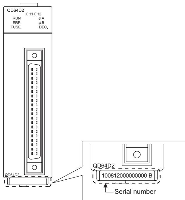
Figure 2.3 Display on the front of the module
