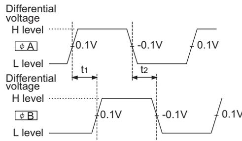
Figure 3.2 Pulse input waveform at 2-phase input 1
