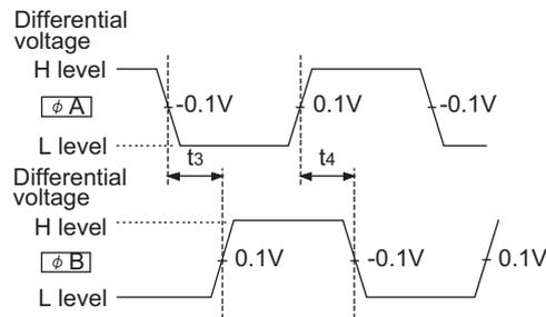
Figure 3.3 Pulse input waveform at 2-phase input 2
