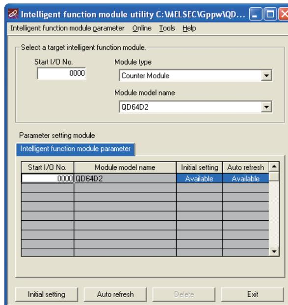
Figure 6.5 [Intelligent function module utility] screen
