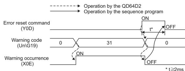
Figure 3.11 Operation of the warning occurrence (X0E)
