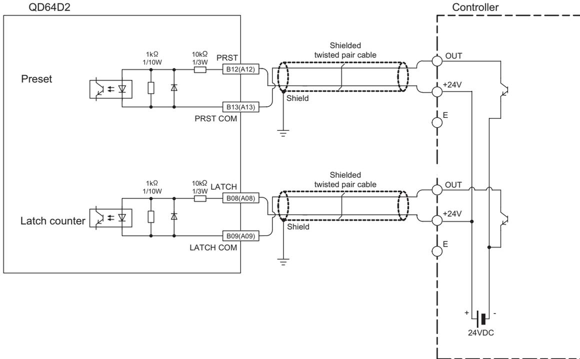
Figure 4.7 Example of wiring with a controller (sink loading type)
