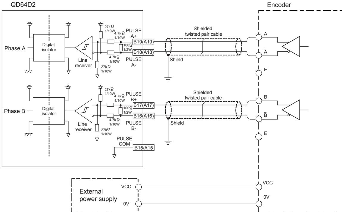
Figure 4.6 Example of wiring with a line driver (AM26LS31 equivalent) encoder
