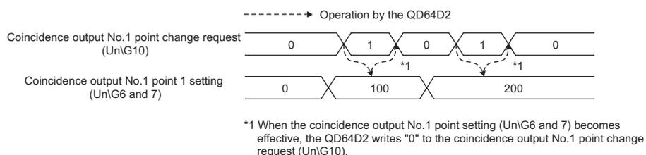
**Figure 3.20 Timing chart for the coincidence output No.1 point setting (Un\G6 and 7) and the coincidence output No.1 point change request (Un\G10)**
