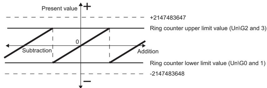
Figure 5.2 Operation image of the ring counter
