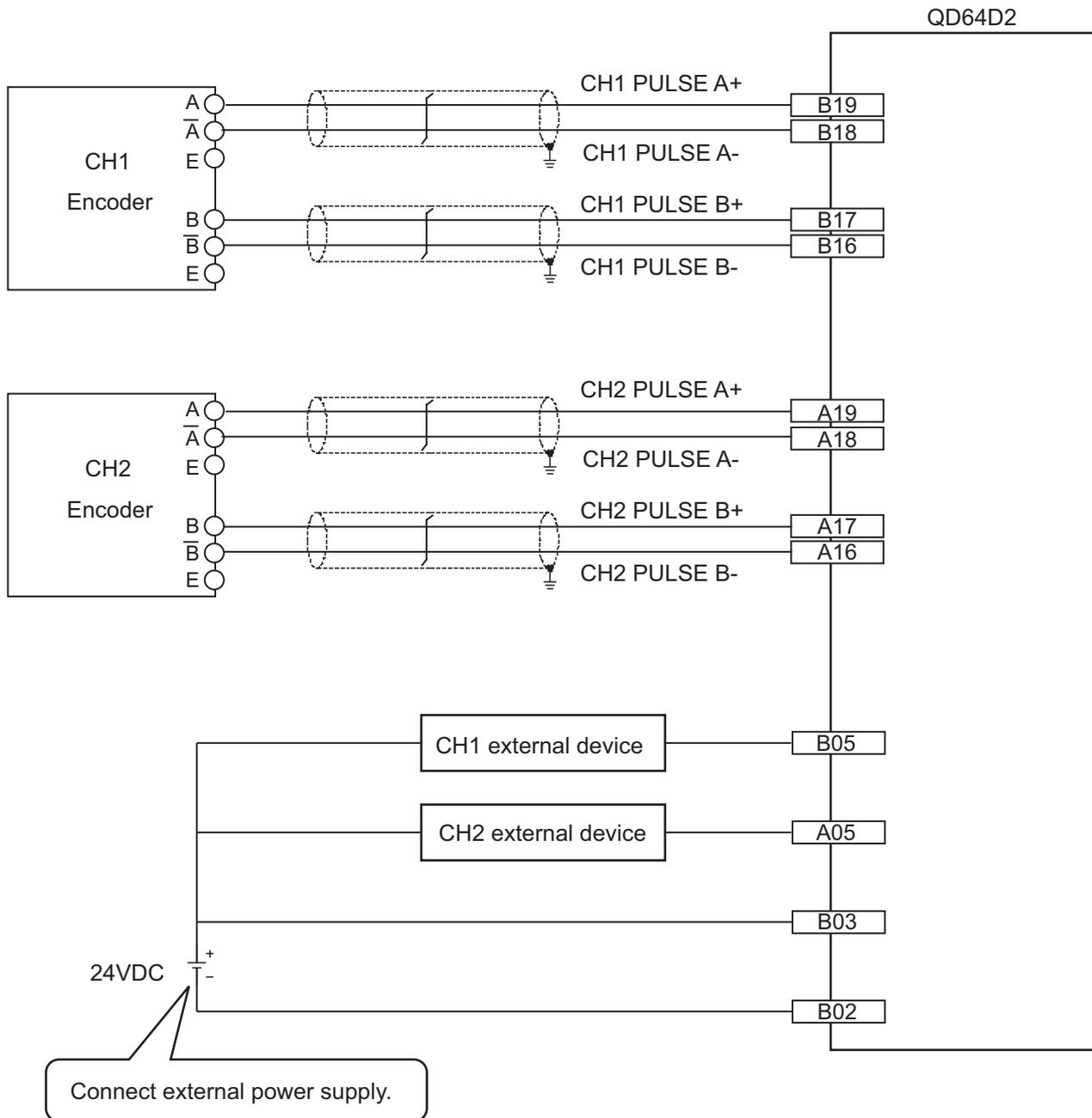
Figure 7.3 Wiring example of the program example
