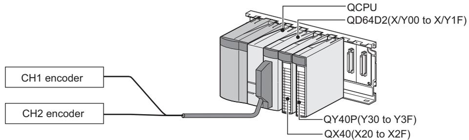
Figure 7.2 System configuration
