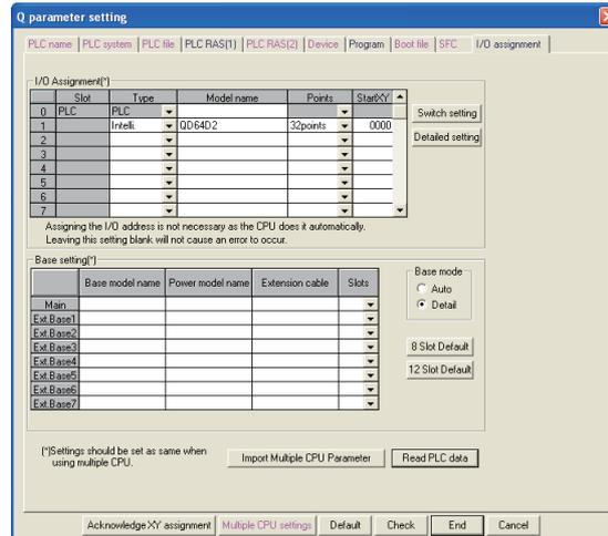
Figure 4.10 Setting example of [I/O assignment]
