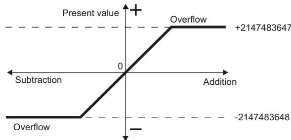
Figure 5.1 Operation image of the linear counter
