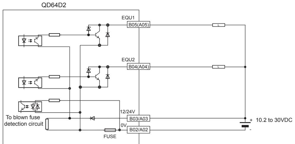
Figure 4.9 Example of wiring with an external output terminal (sink output type)
