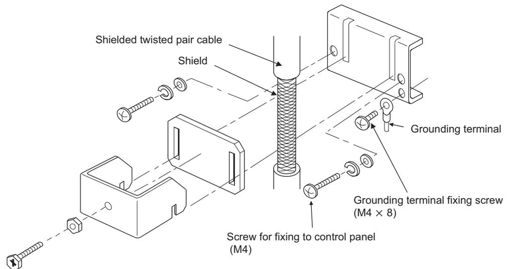
Figure 4.5 Grounding shielded twisted pair cable with the AD75CK
