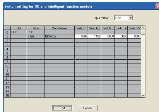
Figure 4.11 [Switch setting for I/O and intelligent function module] screen
