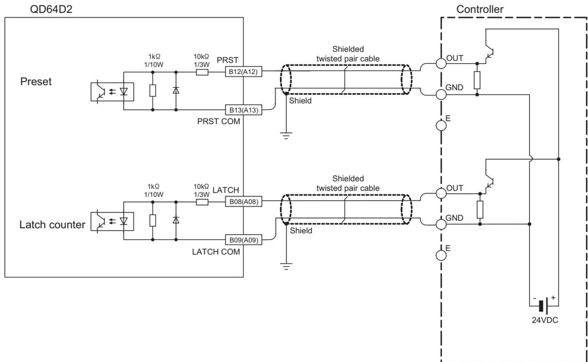
Figure 4.8 Example of wiring with a controller (source loading type)
