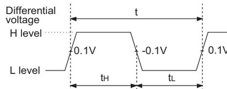
Figure 3.1 Pulse input waveform at 1-phase input
