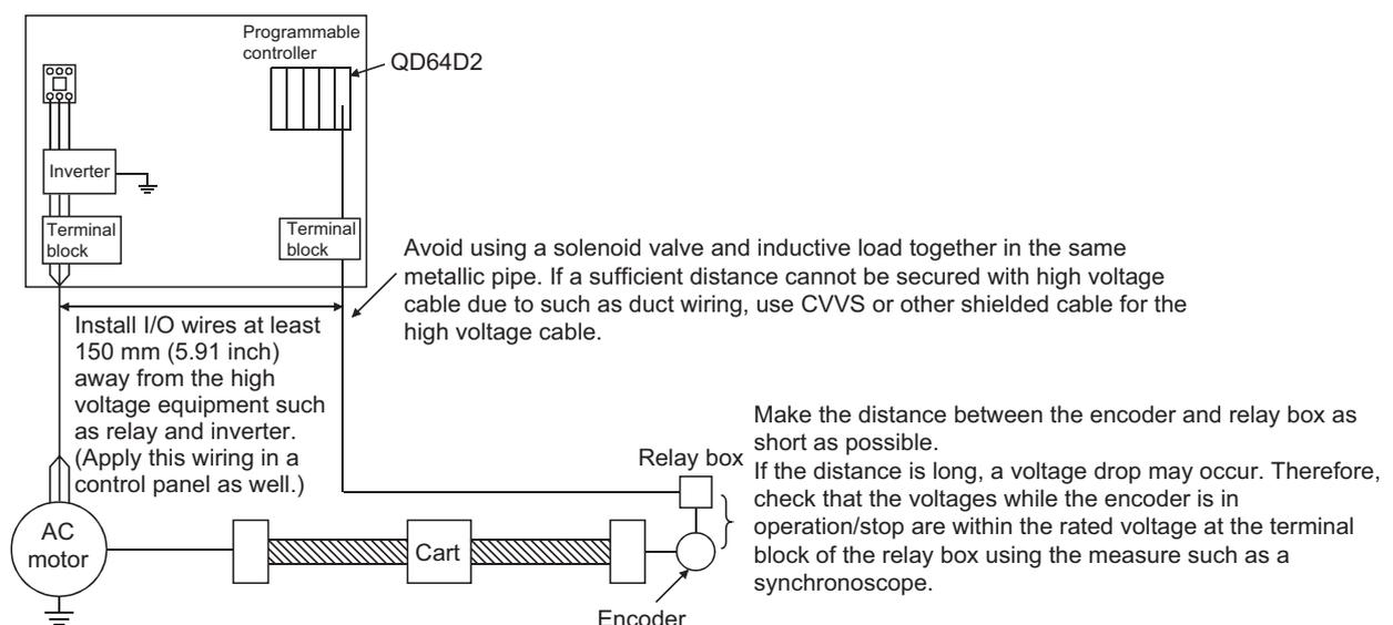
Figure 4.3 Example of wiring for measures against noise
