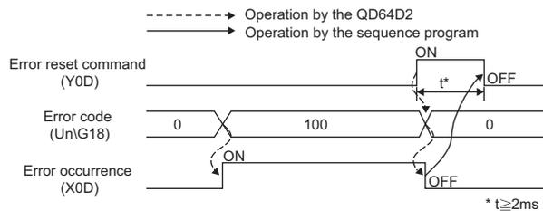
Figure 3.10 Operation of the error occurrence (X0D)
