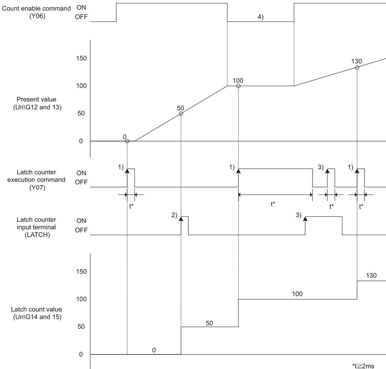
Figure 5.14 Operation example of the latch counter function
