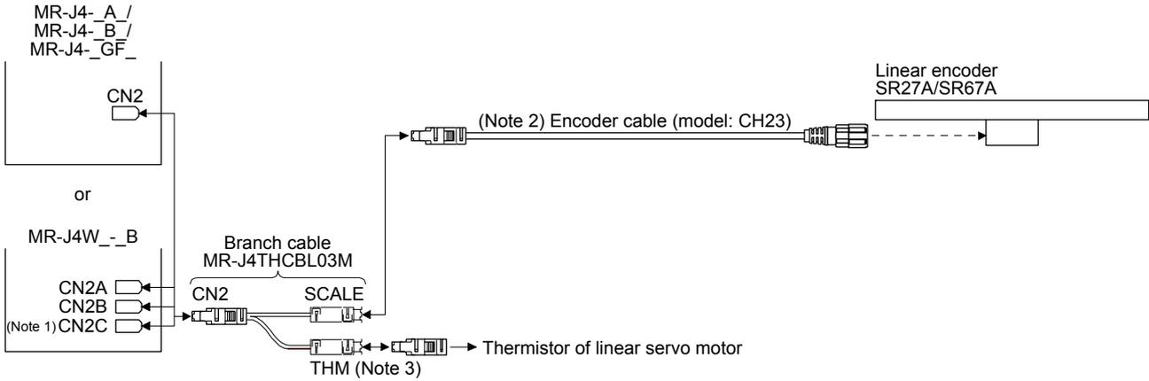
Note 1. The connection to CN2C is for the MR-J4 3-axis servo amplifier. MR-J4 2-axis servo amplifier does not have CN2C.
