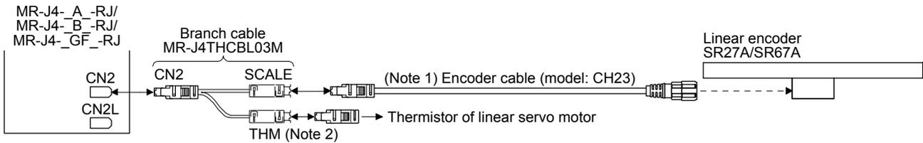
Note 1. This option is manufactured by Magnescale. It should be prepared by the customer.
